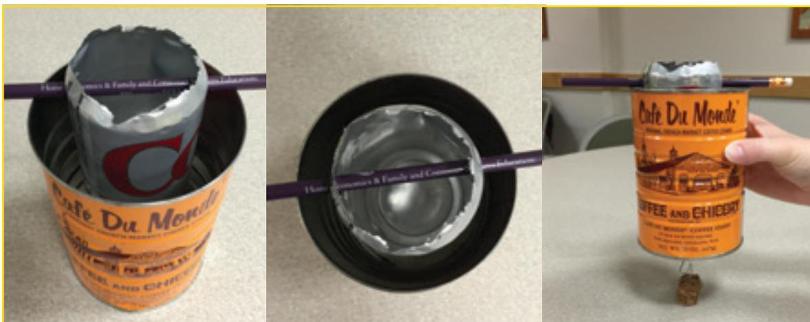
*A bomb calorimeter can be made using everyday items such as a coffee can, soda can, pencil, paperclip and cork.*
