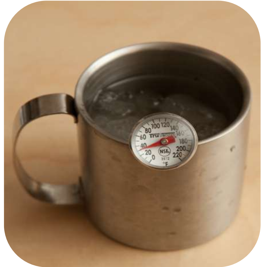
Measuring the Temperature of Ice Water
